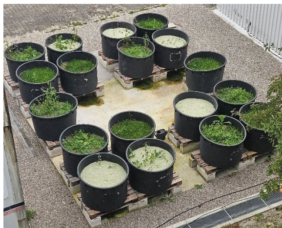
Figure 1 Experimental setup two weeks after application of the zeolite layer
